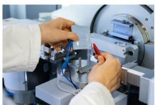
Battery research at JLU: Preparing to analyse the material structure of a battery during operation using X-ray diffraction. Photo: JLU / Rolf K. Wegst
